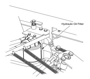
Figure 7-3 Hydraulic Oil Filter
